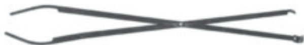
BK-40 Bookcase Equalizer Attaches to the top of the glass door and the back of the bookcase to keep the door centered when it is opened and closed. Steel. Size: 24" Long x 7/16" Wide
