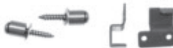
BK-44 Book Case Door Stops and Pivot Brackets Stops mount on frame and pivot brackets mount on door. When the closed door is pulled out, bracket pivots on stop until door is horizontal and can be pushed inside. Includes two stops and two brackets. Steel.
