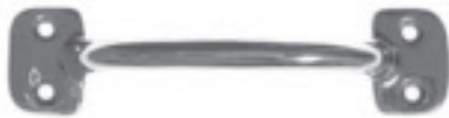
F-9 File Cabinet Handle Polished cast brass handle for file cabinets and other applications. Overall Size: 4-3/4" Long x 1-3/16" High. Screws on 4" centers.
