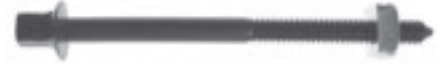
BB-40 Bed Bolt Black steel bed bolt with square nut. Bolt Head: 7/16" Square Overall Length: 6-1/8" Thread: 3/8" x 16
