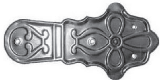
TKW-60 Trunk Slat Clamp Covers wood slats to the top of the trunk and bends over the side of the lid. 2-1/2" Wide x 5-3/8" Long
