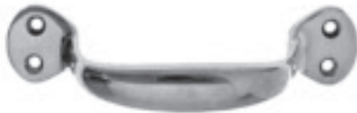
P-142 Cast Brass Handle Polished cast brass handle can be used for doors, drawers, chests or windows. Overall Length: 5-3/4" Center to Center Mounting: 4-3/4"
